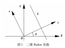
Fig. 1 two-dimensional Radon transform
