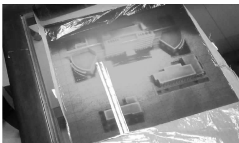
图12 基于逆向衍射技术制作的光子地图板 Fig. 12 Experimental photonic map based on CGH with inverse diffraction
