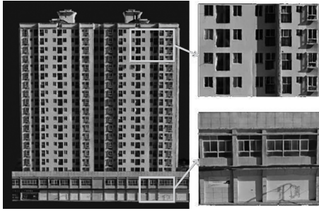
图8 UAV影像点云和LiDAR点云融合建模结果 Fig.8 Fusion modeling results of UAV image point cloud and LiDAR point cloud
